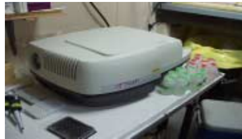
Spectrofluorometer: doesn't work well because of power fluctuations
