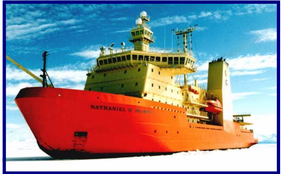
NATHANIEL B. PALMER (Length Overall 308 ft, Beam 60 ft, Draft 21.8 ft, Displacement 6,500 Tons, and 12,700 Shaft Horsepower)
