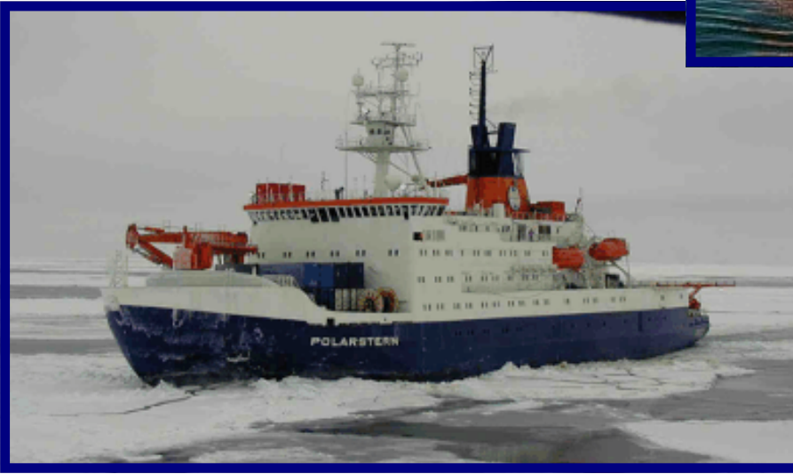
POLARSTERN (Length Overall 387 ft, Beam 82 ft, Draft 34 ft, Displacement 15,000 Tons, and 17,000 Shaft Horsepower)
