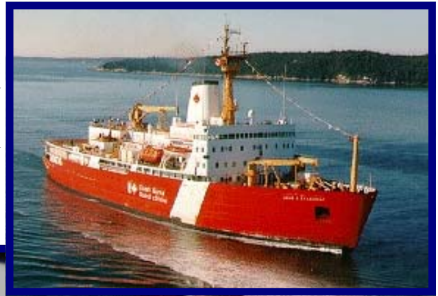
CCG LOUIS S. ST. LAURENT (Length Overall 392.5 ft, Beam 79.9 ft, Draft 31.2 ft, Displacement 14,500 Tons, and 24,000 Shaft Horsepower)
