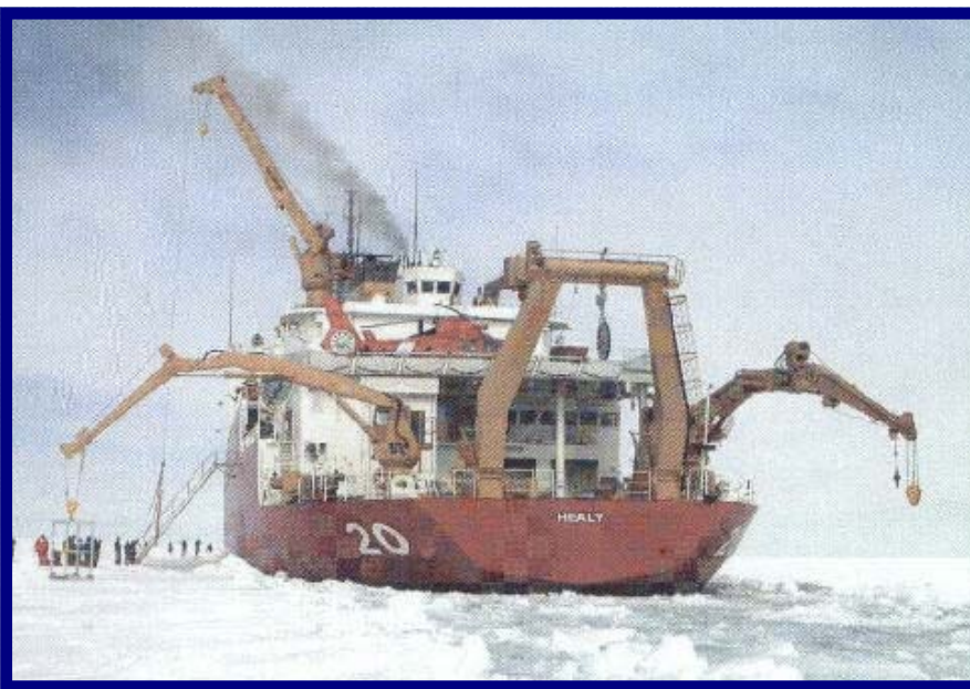
USCGC HEALY (Length Overall 420 ft, Beam 82 ft, Draft 29.3 ft, Displacement 16,000 Tons, and 30,000 Shaft Horsepower)
