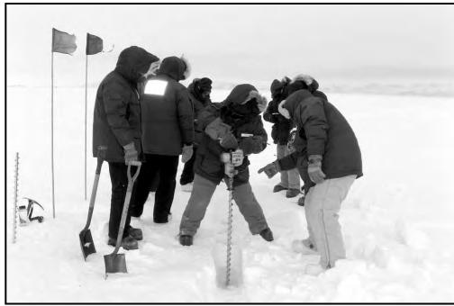
a drill to determine the depth of the annual sea ice near McMurdo Station. Learning how to test ice thickness is required training for anyone driving across the annual sea ice.
