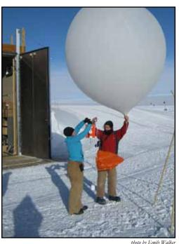
photo by Emily Wa A balloon is launched at Amundsen-Scott South Pole Station to gather clean air samples for analysis by NOAA's Earth System Research Laboratory's Global
