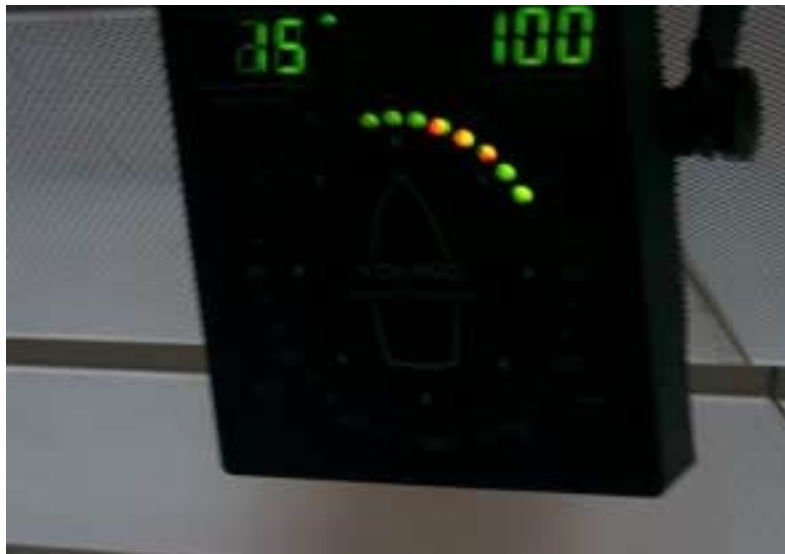
Bridge Anemometer display
