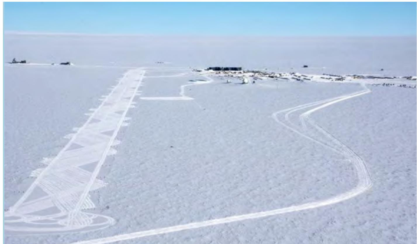
Station Approach. The traverse route curves around the skiway before heading grid-north to the Elevated Station. Source: NSF, Colin Whitmore, Undated.
