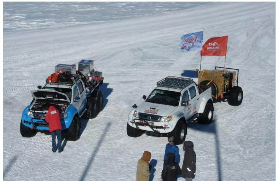
Agile Overland Traverse. Small overland traverse vehicles have been used in Antarctica in the past and may be a cost- and time-saving alternative to field flights in crevasse-free areas. Source: ASC, Unknown.
