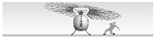
Never approach or leave when the engine and rotors are running down or starting up.
