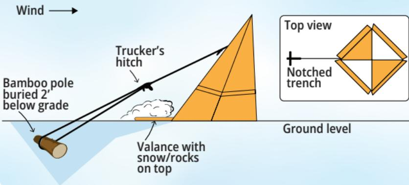
Substrate conditions inform how best to anchor a tent. If the snow or soil surface is **firm** (i.e., hardpacked), hammer in long stakes or sections of bamboo angled slightly away from
